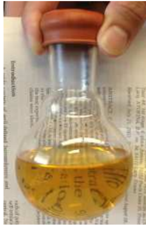
Figure 5.1 Photograph of \text{Fe}_3\text{O}_4/\text{SiO}_2 magnetic nanoparticles prepared via the microemulsion method.
