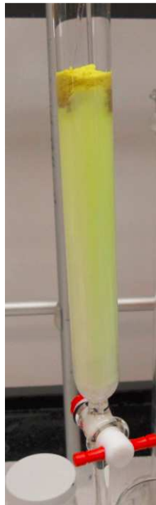
Figure 4.2 Photograph of column purification of polyacid grafted nanoparticles after “click” reaction.
